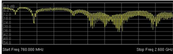
The antenna has a very flat response over all the bands from 700MHz to 3GHz with low noise and can be deployed in single or multiple element arrays to minimize the effects of the hull on receiving the mobile signal.
